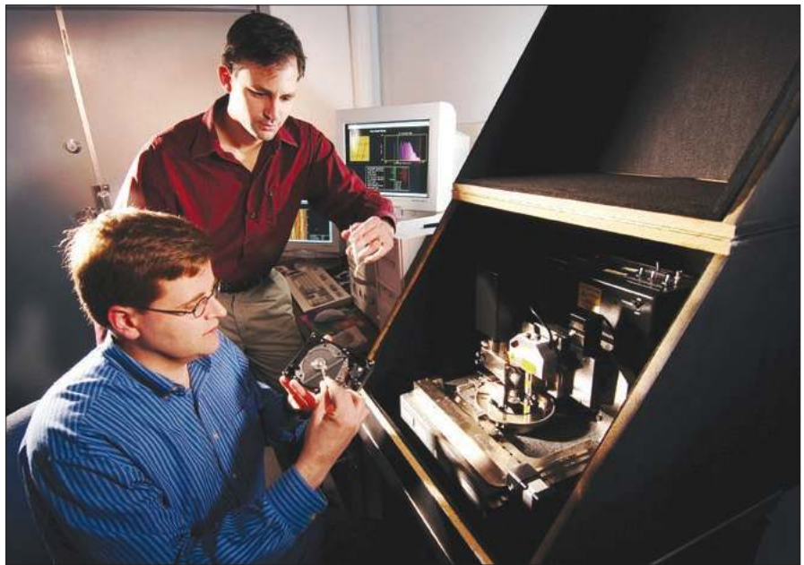
Figure 2 – Researchers image a hard disk drive platter using magnetic force microscopy (MFM) – Georgia Tech Photo: Gary Meek
